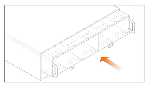
Figure 12: Fan Tray Insertion
