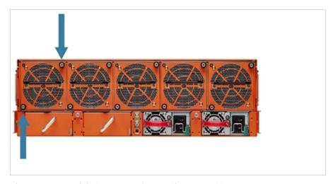
Figure 7: Fan Module Screw Location on GigaVUE-HC3 Rear
