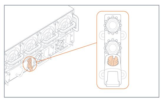
Figure 1: Grounding Lug on Rear of GigaVUE-HC3
