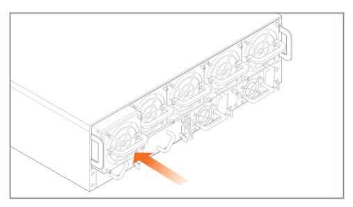
Figure 14: Fan Module Insertion
