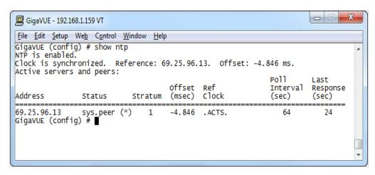
Figure 27: Checking NTP Status and Configuration
