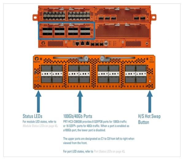
Figure 6: PRT-HC3-C08Q08 Module
