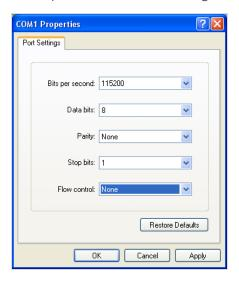
Figure 20: Setting COM Port Properties for the Console Connection
