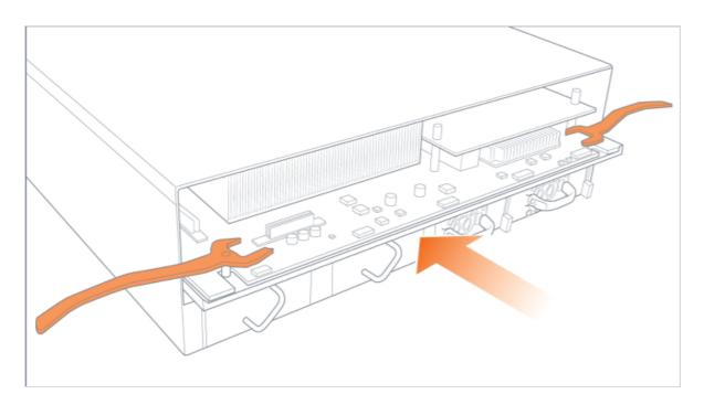
Figure 22: Control Card Insertion
