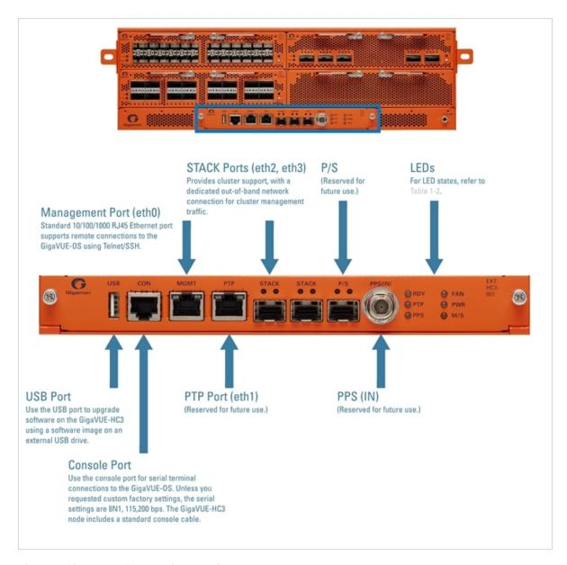
Figure 4: GigaVUE-HC3 Extension Board
