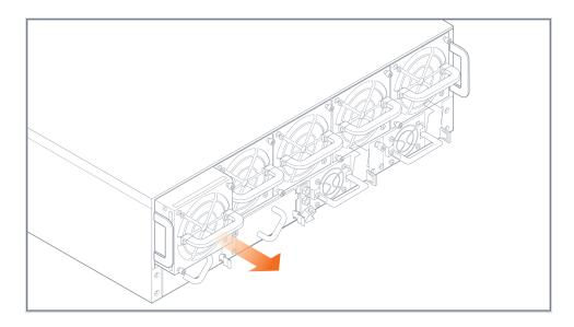
Figure 8: Fan Module Removal
