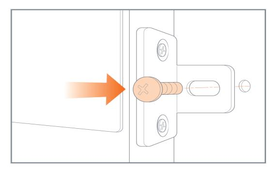
Figure 4: Locking Rack Ear Attached to Rack
