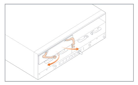
Figure 9: Filler Panel Levers
