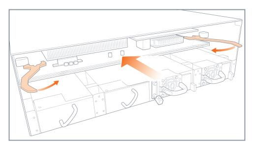
Figure 23: Control Card Ejector Handles
