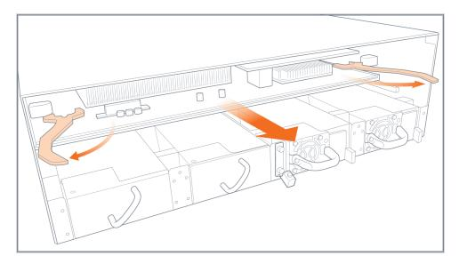
Figure 18: Control Card Ejector Handles
