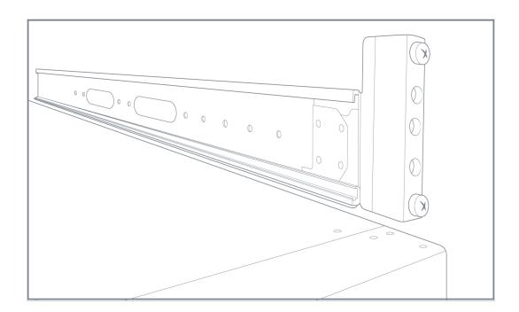
Figure 2: Slide Rail Installed in Four Post Rack
