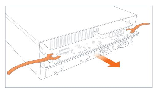
Figure 19: Control Card Removal
