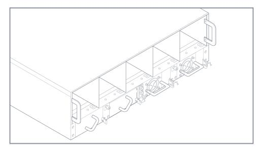
Figure 13: Fan Tray Inserted
