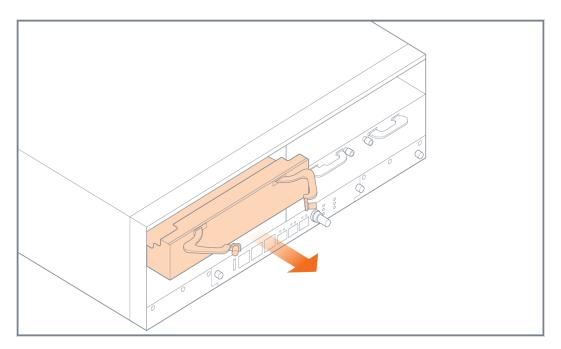
Figure 10: Filler Panel Removal
