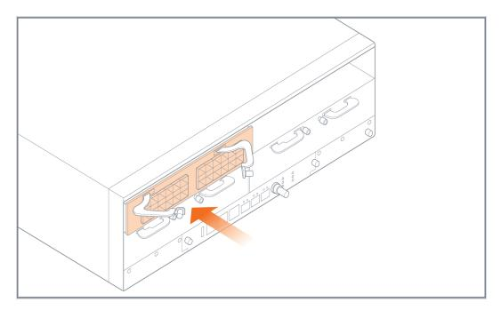
Figure 12: Module Insertion
