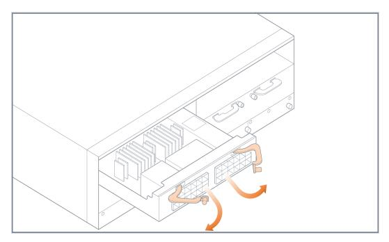
Figure 11: Module Levers
