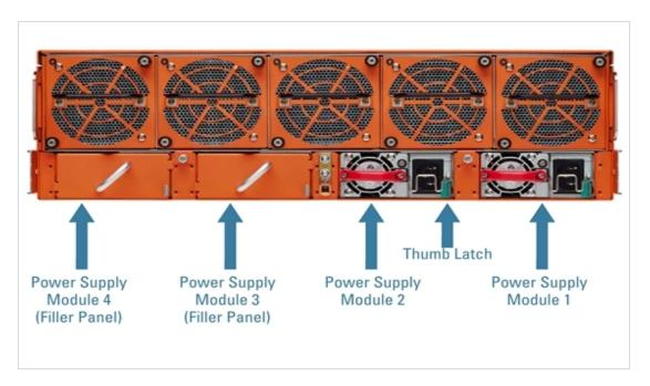
Figure 5: Power Supply Modules (AC Version Shown)
