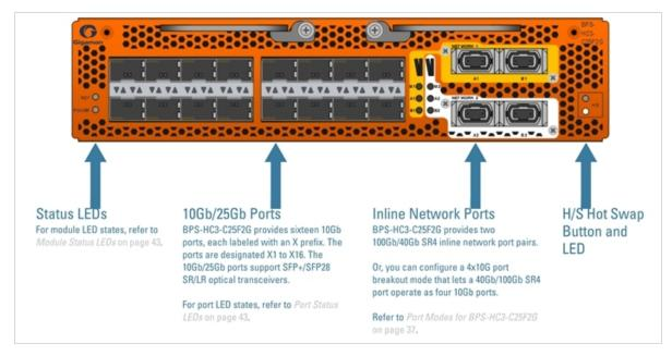
Figure 9: BPS-HC3-C25F2G Module
