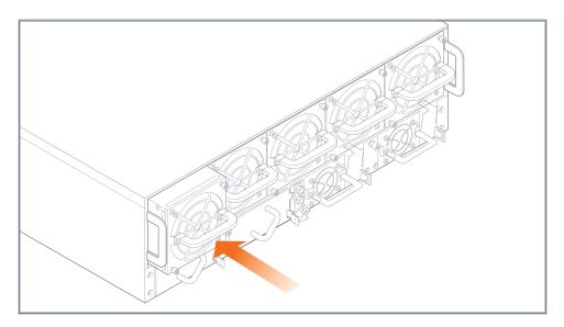
Figure 9: Fan Module Insertion
